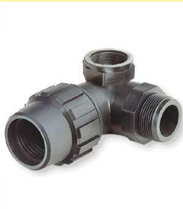
CODO FITTING 3 SALIDAS (1 FITTING - 1 R/HEMBRA - 1 R/MACHO) P.E. 3 OULETS FITTING ELBOW (1 FITTING - 1 FEMALE - 1 MALE) P.E. COUDE PRESSION 3 SORTIES (1 PRESSION - 1 FILETÉ - 1 TARAUDÉ) P.E. JOELHO FITTING 3 SAIDAS (1 FITTING - 1 R/H - 1 R/M)
